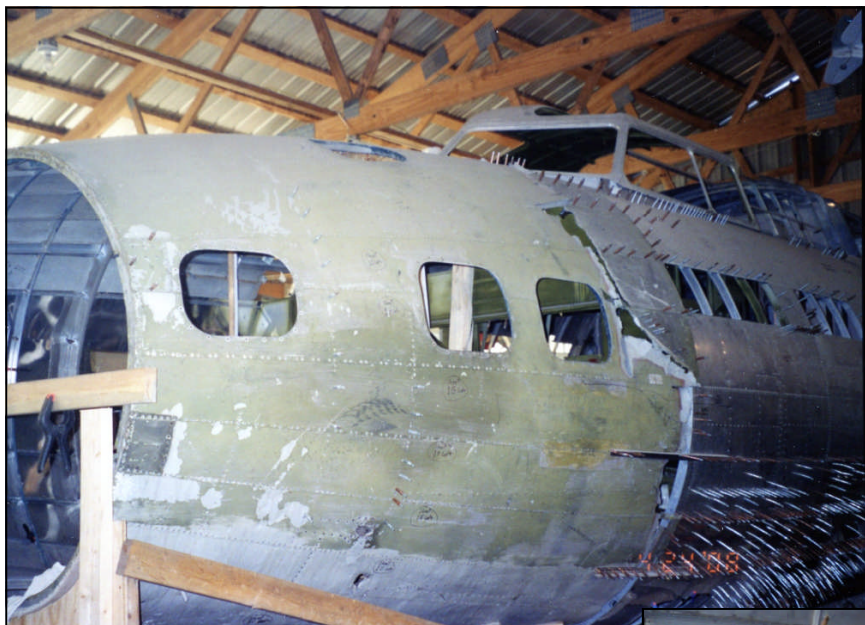
Damage Done With an Axe
