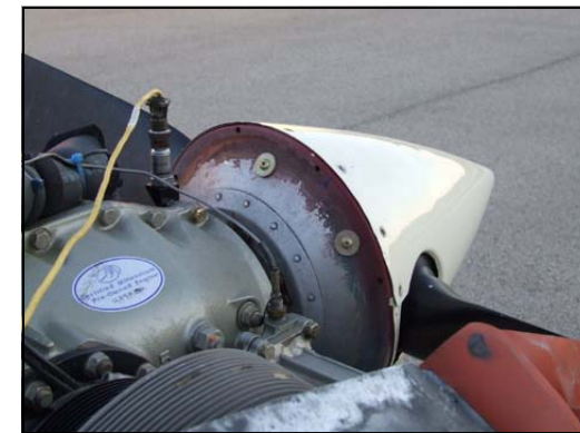
Pictures #7, #8—Permanent balance weight attachment.
