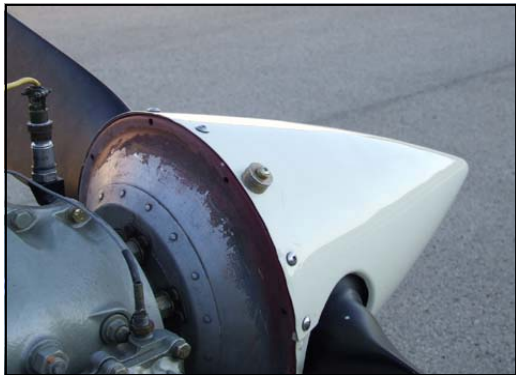
Pictures #7, #8—Permanent balance weight attachment.
