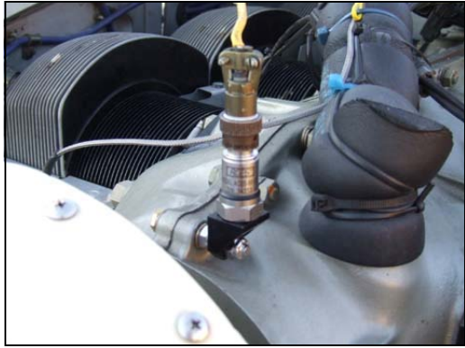
Pictures #3,#4—Taking a reading of the out of balanced condition of the prop.
